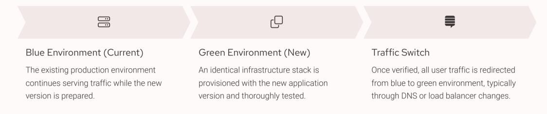
This method minimizes deployment risk with zero downtime and enables immediate rollback by switching traffic back to the blue environment if issues arise. The primary consideration is maintaining two complete environments simultaneously, which increases resource costs.
